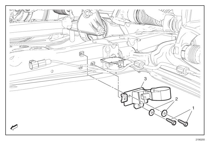
If the front headlamp leveling sensor (3) has been found to be the cause for the customer concern, the leveling sensor must be replaced.
