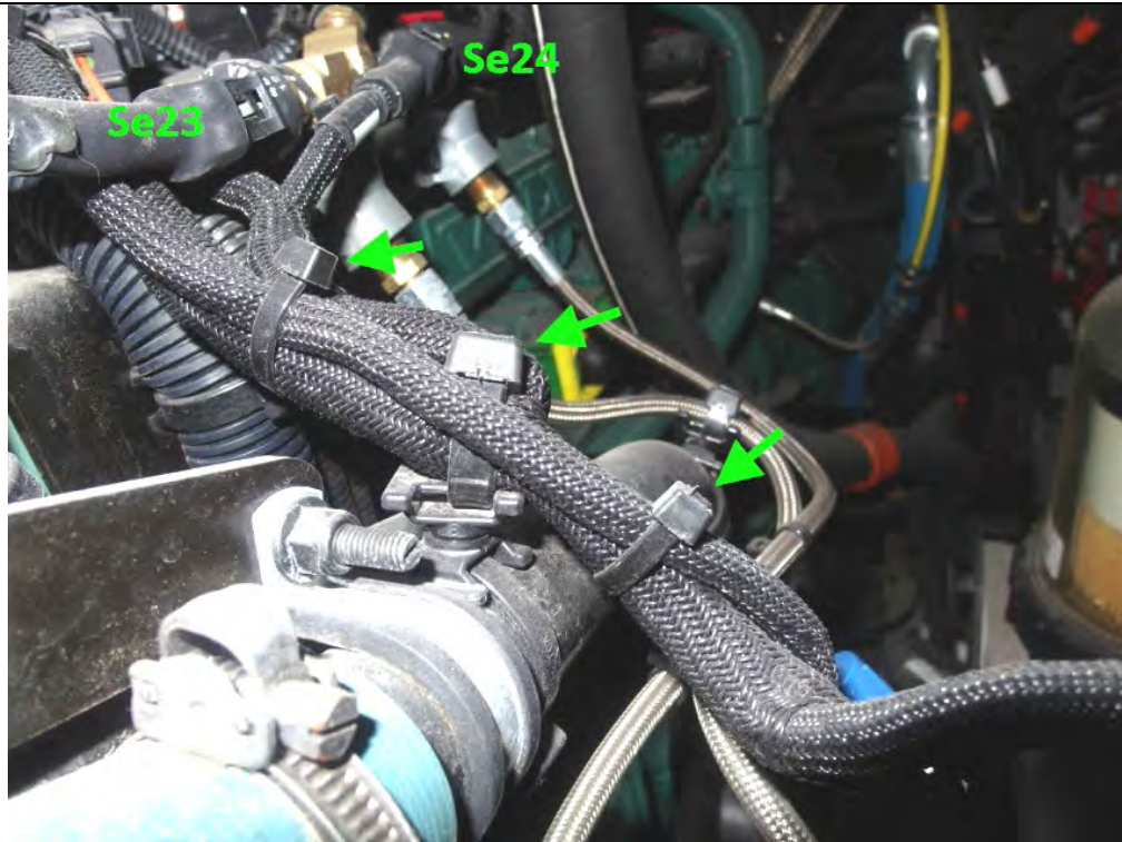
ATTACH THE EXCESS LENGTH OF CABLE ALONG MAIN STRAND OF HARNESS AS SHOWN- NYLON TIES LOCATION SHOWN BY ARROWS
