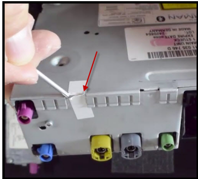
Figure 7. Break the white warranty seal.
