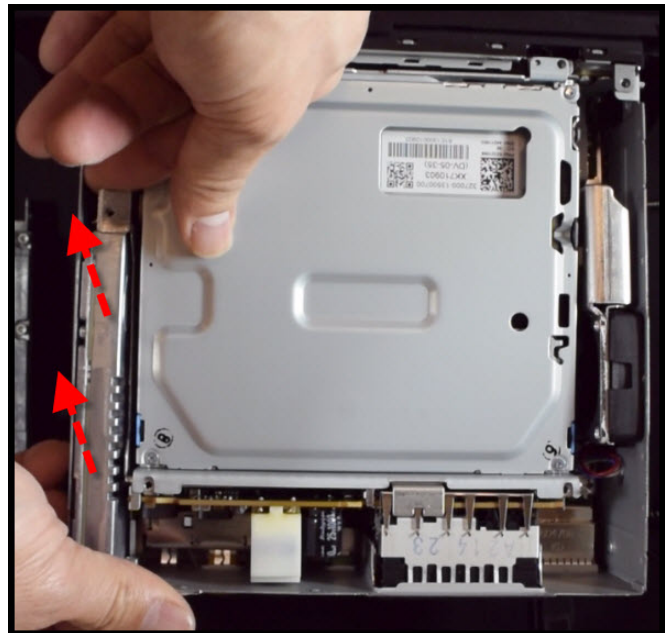
Figure 13. Lift up on both ends of the telephone module as indicated by the red arrows.
