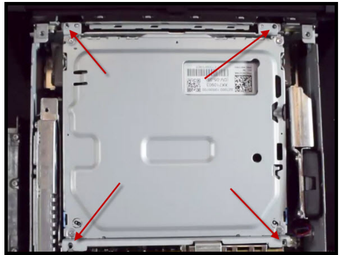
Figure 11. CD drive mounting points are now free.
