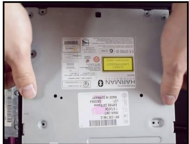
Figure 7. Pry top cover off with fingers.
