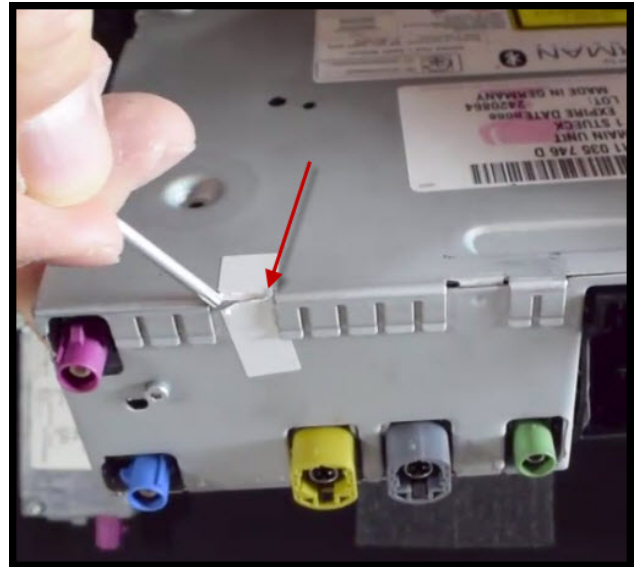
Figure 6. Break white warranty seal.
