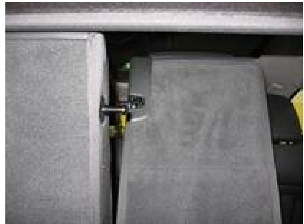
Figure 2. Armrest lock striker pin.
