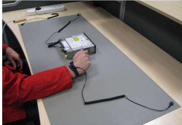
Figure 6. ESD Complete Setup.
