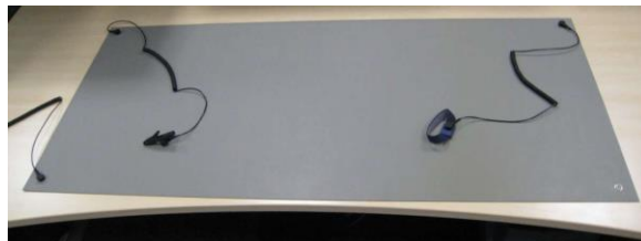
Figure 3. ESD Work Surface.
