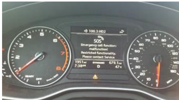
Figure 1. SOS warning in instrument cluster.
