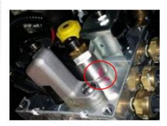
7. To allow a socket to be placed over the fuel pressure regulator housing for removal, it will be necessary to loosen the air solenoid retaining nut located above the fuel pressure regulator and rotate slightly. Refer to the photographs below, which show a view of the atomizer from above, for reference. The atomizer pictured has been removed from the vehicle for clarity.
