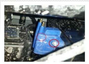
**3.** Remove the combustion chamber inlet temperature sensor and reposition it to allow for sufficient clearance to remove the atomizer cover. The harness can be left connected.
