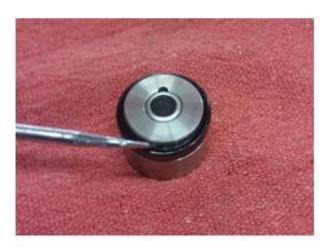
**11.** Lubricate the piston and the new U-cup seal lightly with silicone grease to ease installation. Slide the new U-cup seal over the piston, ensuring the cup faces away from the piston as shown.
