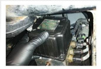
21. Replace the four screws retaining the atomizer cover and tighten to the specified torque.
