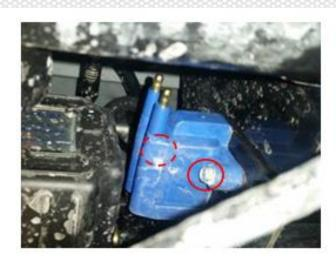
23. Reconnect the ignition wires to the ignition coil.
