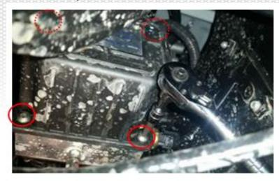
5. The atomizer cover can be removed by first rotating the cover over into the space previously occupied by the ignition coil. Make certain the wire harness grommet releases from the front side of the cover. The cover can then be moved downwards toward the combustion chamber and again rotated to remove. This is a very tight fit, but the cover can be removed without force once it is positioned correctly.
