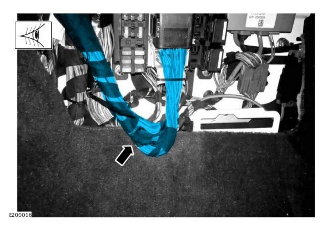
**4.** Position the wiring harness behind the floor carpet as illustrated.
