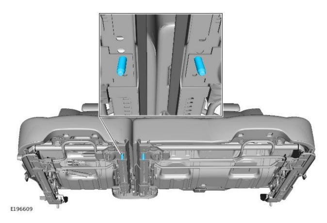
3. NOTE: The existing metal washers should still be installed.
