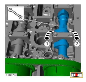
**4.** Refer to intake camshaft VCT actuator (see TOPIx Workshop Manual section 303-01A / 303-01B: Engine - GTDi 2.0L Petrol - Variable Camshaft Timing Actuator).
