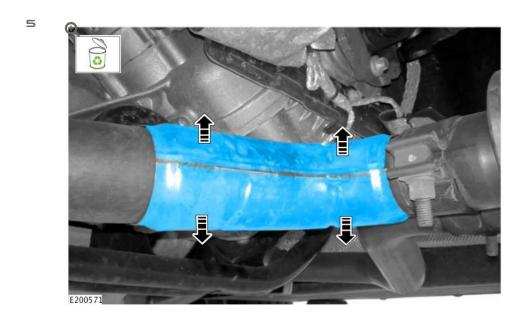
Remove and discard both the upper and lower sections of the heat shield.
