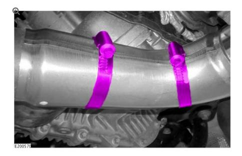
Install the two inner hose clips over the two indented lines on the new heat shield.
