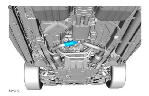
Identify the location of the loose exhaust heat shield.
