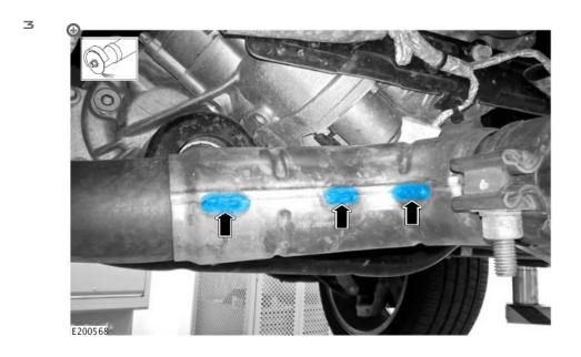
Using a suitable tool, remove the three welds from the inside of the bend on the exhaust heat shield.
