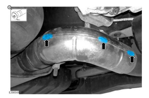
Using a suitable tool, remove the three welds from the outside of the bend on the exhaust heat shield.
