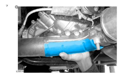
Install the lower section of the new heat shield onto the downpipe.
