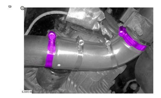
Install the two outer hose clips on the smaller diameter section of the heat shield.
