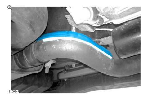
Install the upper section of the new heat shield onto the downpipe.
