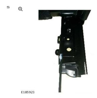
Push the NyoGel® 774 (or equivalent Polyalphaolefin based, silica thickened, synthetic hydrocarbon grease, with a viscosity index of 274) grease into both seat tracks with a new cable tie.
