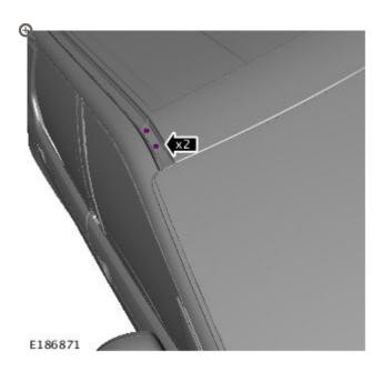
Tighten the two nuts below the roof moulding.
