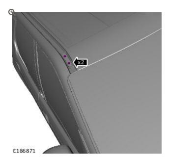
Fully loosen the two nuts below the roof moulding.
