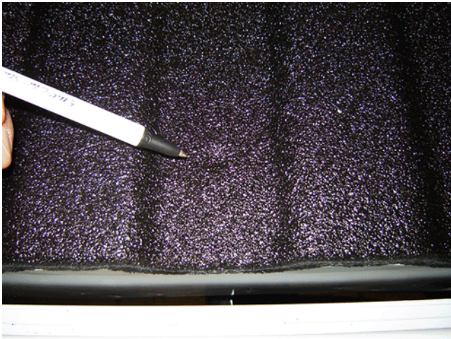
Spot weld under bed liner example
