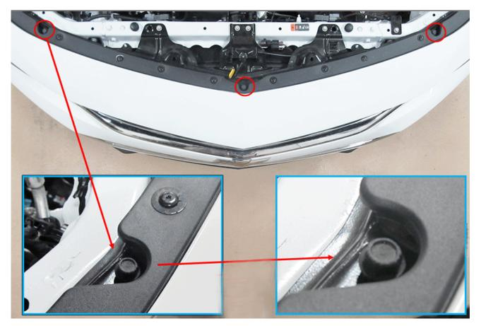
**Important:** DO NOT attempt to tighten or otherwise move these three fasteners. These fasteners are part of the front fascia support bracket which have a preset gap by design and the plant does not adjust these fasteners when they install the fascia assembly to the car.
