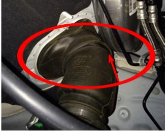
2. Remove the intermediate steering shaft boot (seal) (inner). Confirm that the bearing is properly seated inside the rubber boot. Refer to *Intermediate Steering Shaft Boot Replacement (Inner)* in SI.
