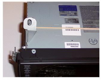
• The illustration above shows a radio with damaged mounting tabs.
