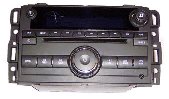
• The illustration above shows a radio with a cracked display window.
