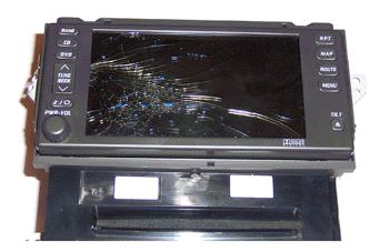
• The illustration above shows a navigation radio with a cracked display window.
