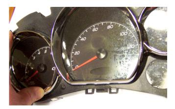
• The illustration above shows an IPC with chemical damage to the lens.
