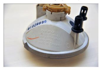
This fog lamp was returned for retaining moisture. As you can see it is marked with the Depo brand (it is also called out on the front lens).
