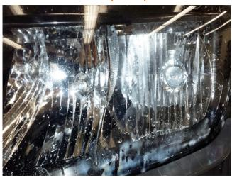
Numerous & Various Size Drops of Water Collecting on the Inside Surface of the Lamp Lens After the Vehicle Has Been Exposed to Rain or a Car Washing Environment
