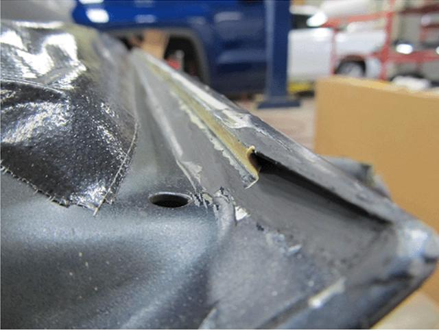
13. Using a squeegee, force the sealer into the open joint area.
