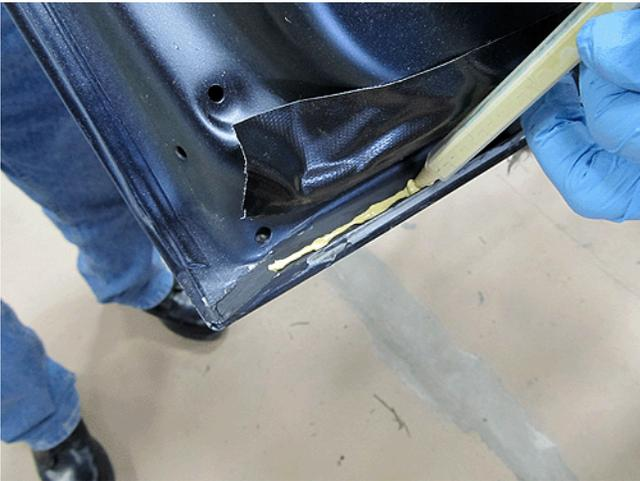
12. Using a small tip opening, apply a small bead of seam sealer such as \*LORD Fusor® 806HD (beige) = 10.5 oz (310.5 mL) or the equivalent to the open joint area.
