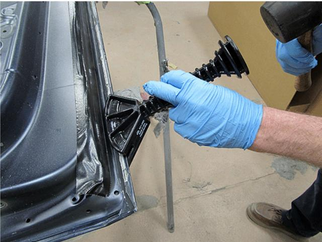
14. Close the hem flange using the flange closing tool.
