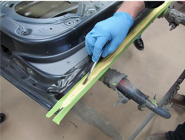
Use a small brush to finish the area, the sealer will self level to remove any brush marks.
