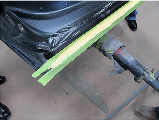
16. Apply a bead of \*LORD Fusor® 806HD (beige) = 10.5 oz (310.5 mL) or the equivalent, as shown to completely seal the hem flange.
