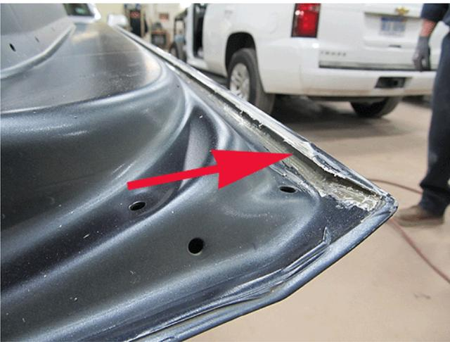
4. Using the appropriate (left or right hand) flange opening tool, open the flange as shown.
