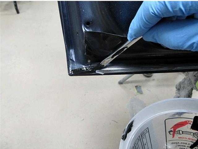
10. Apply a light coat of \*Lloyds Kryptonite Metal Treatment P/N 36502 with a small brush as shown. This first coat should flash in approximately 3-5 minutes.
