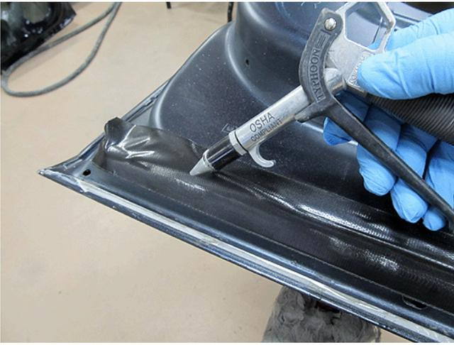
8. Using a water dampened clean towel, remove any residue and dry the affected area. Dry the repair area completely using an air hose to blow dry the frame.
