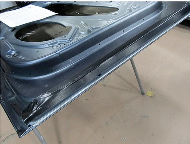
5. Protect the adjacent area with cloth protective (duct) tape.
