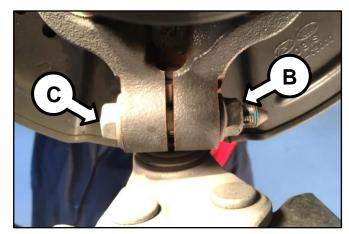
4. Remove the two (2) nuts and one (1) bolt anchoring the ball joint to the lower control arm.
