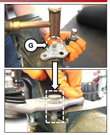
Secure the ball joint to the lower control arm and reinstall the two (2) nuts (H) and bolt (I).
