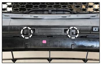
4. Remove the air intake grill by carefully pulling at each end (left and right) with an upward motion, while simultaneously pushing down on the bumper cover. Unseat the air intake half way at one end and continue at the other end to remove the grill completely.
