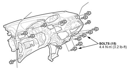
8. Lift up on the dashboard to release it from the guide pins, then carefully remove the dashboard through the front door opening.
