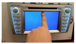
8. Touch Calibration Screen is displayed. Follow the calibration prompts by placing your finger in the center of the cross hairs.
