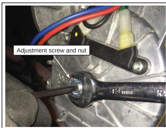
Figure 9 - Axial Play Adjustment
