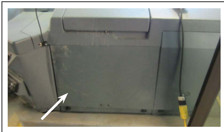
Figure 1 - Typical Front Dash Access Panel
