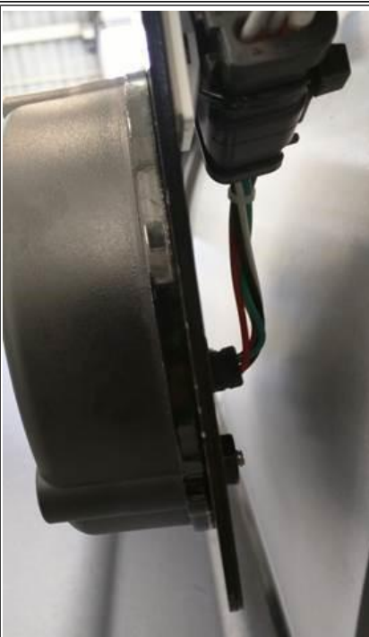
Figure # 2 : VORAD side sensor spacer (Installed)
