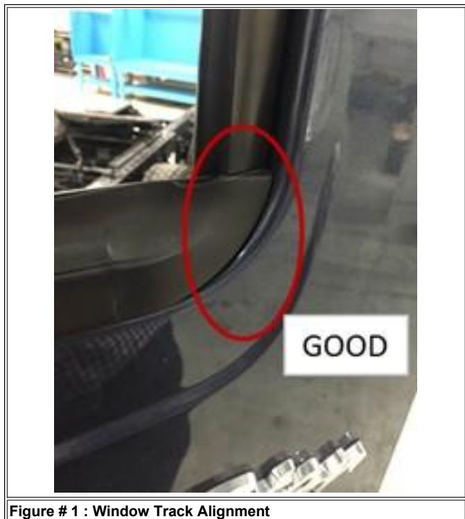
Figure # 1 : Window Track Alignment
