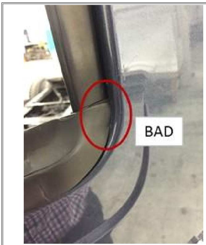
Figure # 2 : Window Track Alignment
