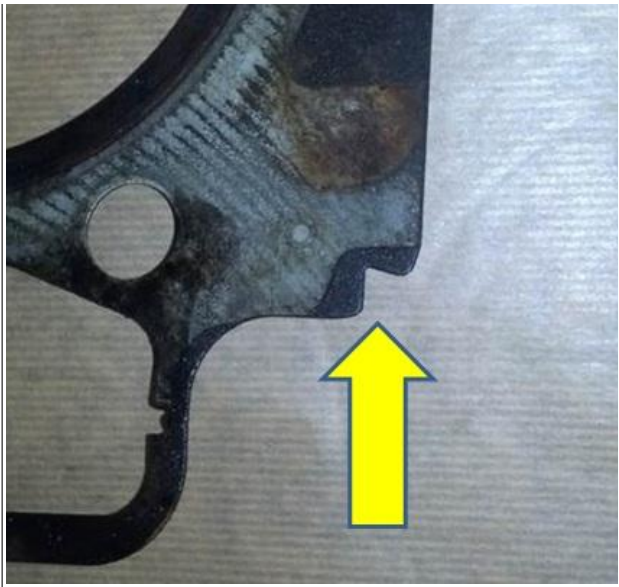
Figure 3: 13L Head Gasket
