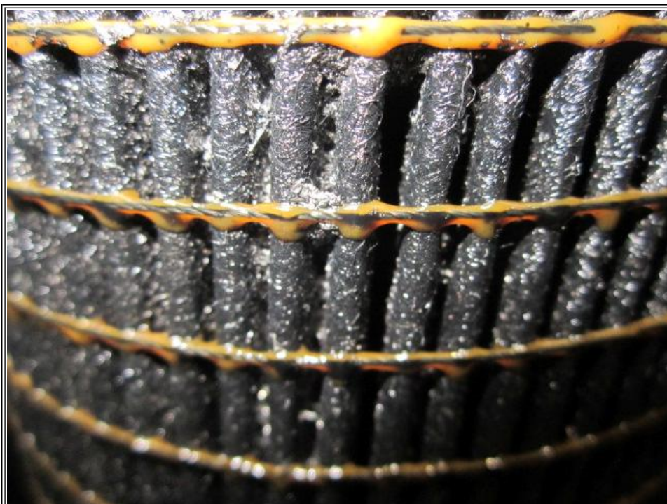
Figure 1: Oil filter with metal shavings present
