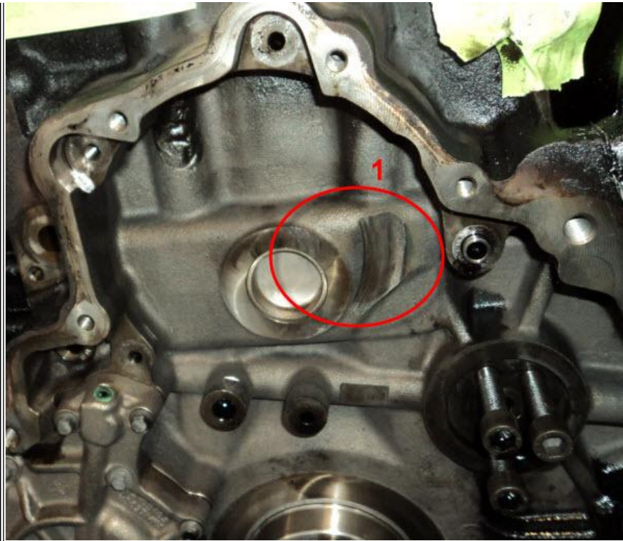
Figure 7: Acceptable engine block wear
