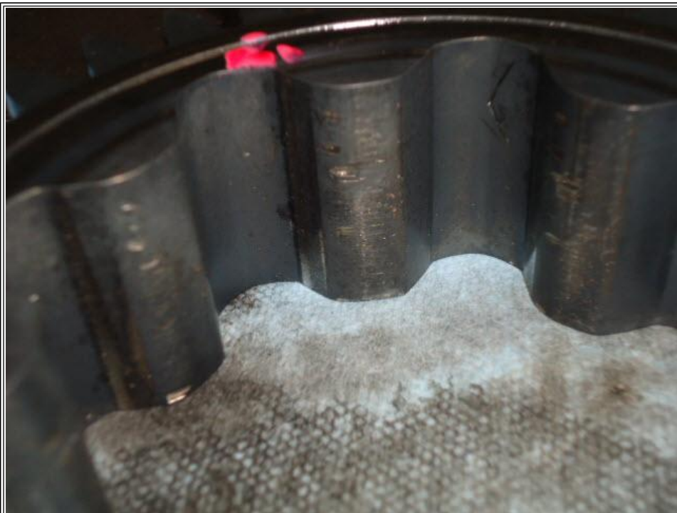
Figure 5: Damaged oil pump/gerotor
