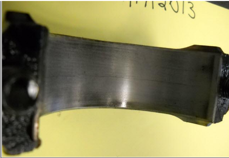
Figure 2: Good bearing - reusable
