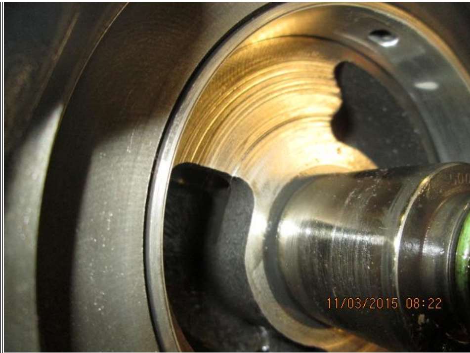
Figure 6: Acceptable engine block wear behind oil pump
