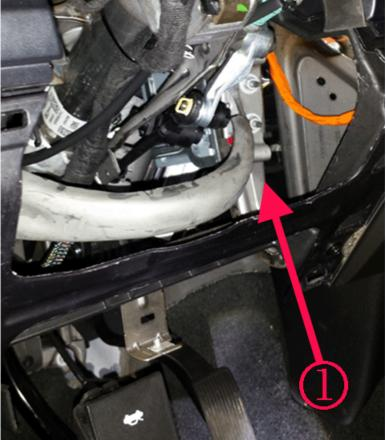
Inspect the power inverter module for possibly moving slightly against mounting bracket and creating the noise.
