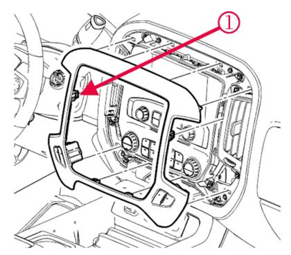
This will require an application of BRS flocking tape on ten retainers (one strip @ 1" x 10"). Two sheets should repair 16 vehicles.
