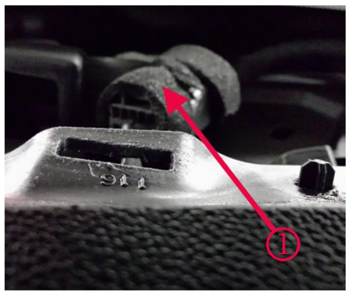
Apply foam tape to all mounting hooks in the front of the defroster grill # 1 and apply a strip of foam tape along the edge of the grill to isolate the grill from the dash #2.
