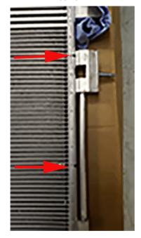
If there a difference of more than 10 degrees F top to bottom, replace the condenser. Reference the Parts Information section below.
