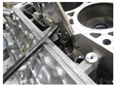
Note: Be sure not to pry on the sealing surface of the block.
