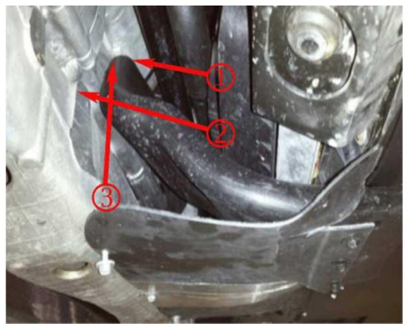
7. Once the part is riveted into place, dry fit to the car to make sure enough of the duct is cut to allow it to sit between the steering motor(1) and the lower rack (2).
