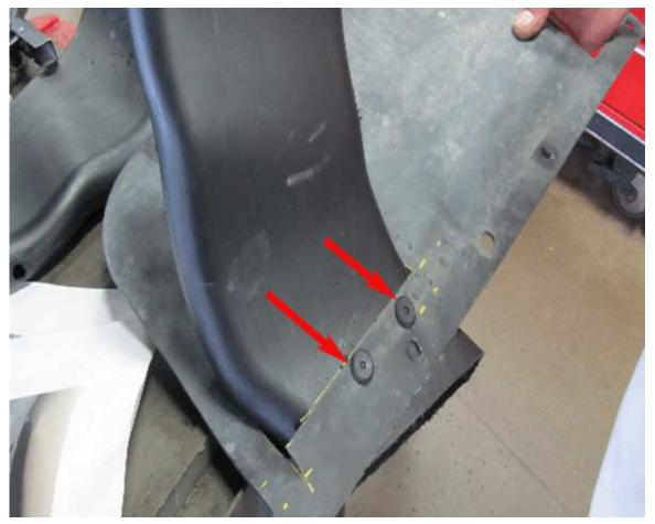
6. Place the cut duct into the slot. Make sure it comes out of the slot 25.4 mm (1 in). Using a 17/64" drill bit, drill 2 holes through the deflector and duct and rivet together.
