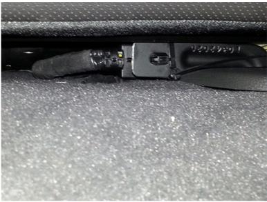
4. If after performing the above suggestions and the 60% side of the seat does not fold down even with the 40% side, remove the two rubber bumpers
