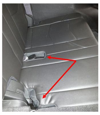
3. If the seat harness, under the left side of the 60% seat, is not properly routed (1) or the seat connector is not properly attached to the bracket, this may obstruct the seat from moving down flat on the floor (2).
