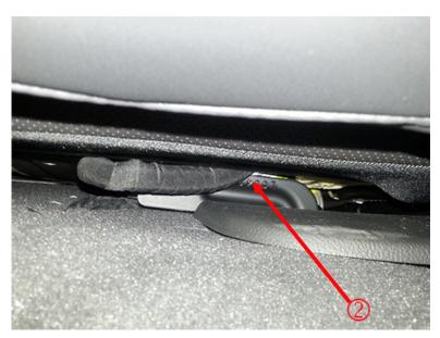
If the seat harness is out of position, reroute the seat harness as shown below (3) and properly secure the seat connector to the bracket as shown (4). The use of a zip tie may be necessary to hold the connector in place. After making repairs, power fold the 3rd row seat down and make sure the seat bottom is not contacting the seat harness, connector or bracket as shown below.
