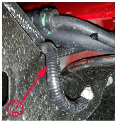
If no water intrusion or corrosion is found in the connector, remove the tape from the G400 conduit and continue with published diagnostics. Please note in the repair information if there was water in the conduit.
