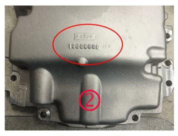
If the pan has raised marking in this location the pan will need to be repaired (see repair procedure). If markings are not present vehicle is good and can be released.
