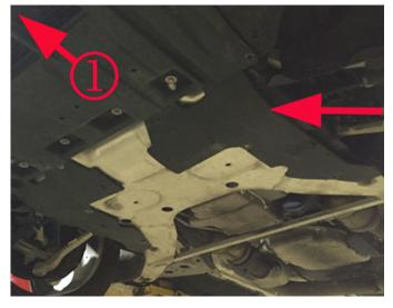
Pan part number will be about 6" behind the crank pulley, just rearward of the first "step up" surface.
