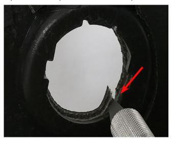
3. On the back side of the trim pad, use a utility knife and trace the cavity to cut away the excess material.
