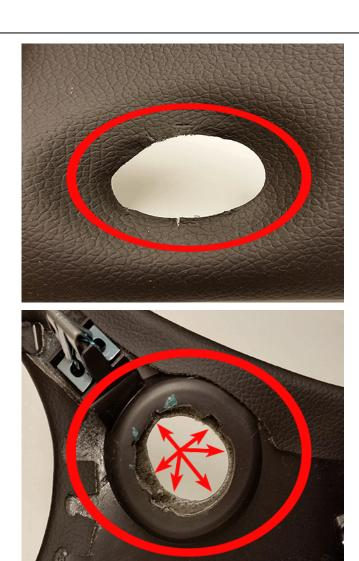
This condition may be due to excess material in the ignition and start switch cavity.
