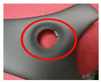
Note: Once the excess material has been removed, the opening for the switch will look rounded as opposed to an oval shape.
