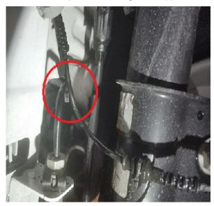
When installing the new wiring harness, allow the wheel speed sensor harness to run above the top side of the brake line as indicated in the picture.
