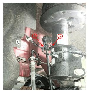
Note: Only replace the speed sensor harness that has been found to be damaged or installed incorrectly.
