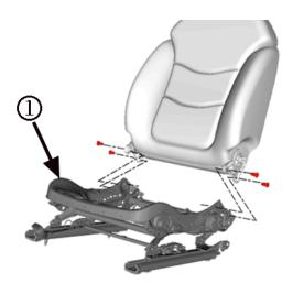
Replace the front seat cushion frame (1) on the affected seat. Refer to Driver or Passenger Seat Cushion Frame Replacement in SI.
