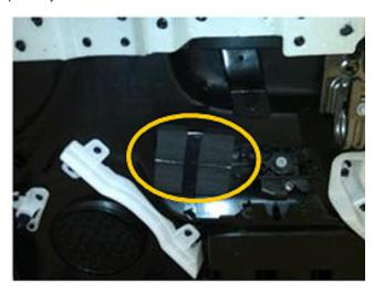
• If the rattle is caused by the water shield, install two 100 mm (4 in) long layers of 1" x 9/16" adhesive backed foam shim stock such as \*Kent Industries Part # P46515 or the equivalent, to compress the water shield as shown. Confirm any added foam does not interfere with the window or door lock operation.
