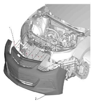
1. Remove the front bumper fascia (2). Refer to Front Bumper Fascia Removal and Installation in SI.
