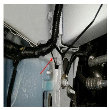
**Note: Do not** over tighten the tie straps. Only tighten the straps enough to allow for proper clearance between the horns, bracket, and the wiring harness.
