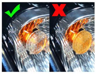
If this condition exists, replace the headlamp(s) that have the amber colored diffuser/lens. Refer to Headlamp Replacement in SI. **Note:** Both headlamps should have clear diffuser/lens for the turn signal inside the headlamp assembly. Only the bulb should be amber in color. All service parts contain a clear/diffuser/lens.
