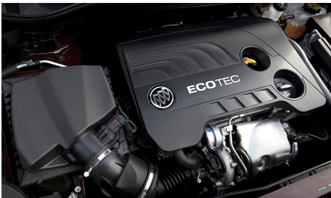
Typical underhood view of the Cascada 1.6L turbocharged engine.
