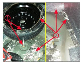
Verify the condition, then remove trunk trim as necessary to inspect the trunk floor and spare tire for evidence of rust (1) or mold/residue (2).
