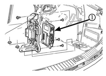
When water damage is evident, replace the radio speaker amplifier (1). Refer to Radio Speaker Amplifier Replacement in SI.
