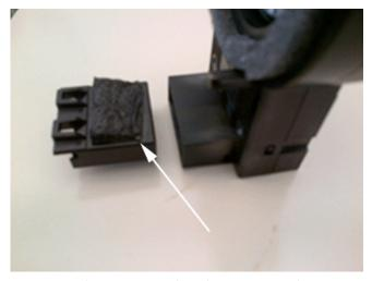
2. Add a piece of Adhesive Back Shim Stock the width of the connector to the flat surface on the male connector. This provides support to the connector to keep it from moving up and down.
