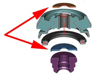
**Important:** Unlike the previous design, the top and bottom washers are now unique. The top washer is Part Number 92273396 and the lower washer is Part Number 92421239 and must be oriented with the flat surface facing upwards.
