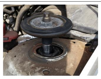
This may be caused by premature wear within the front strut mount.
