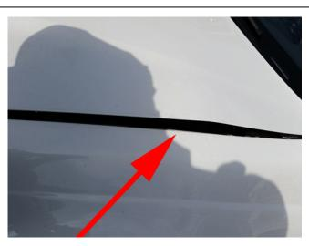
Some customers may comment that the front strut shaft has come free from the strut mount and made contact with the vehicles hood.
