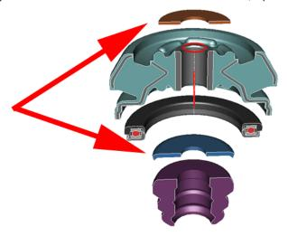
Important: Unlike the previous design, the top and bottom washers are now unique. The top washer is Part Number 92273396 and the lower washer is Part
