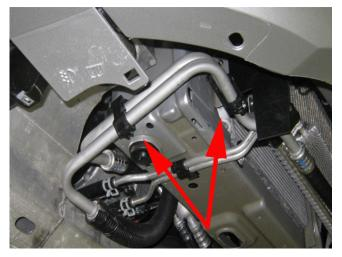
The clips should be installed in the approximate location shown above.
