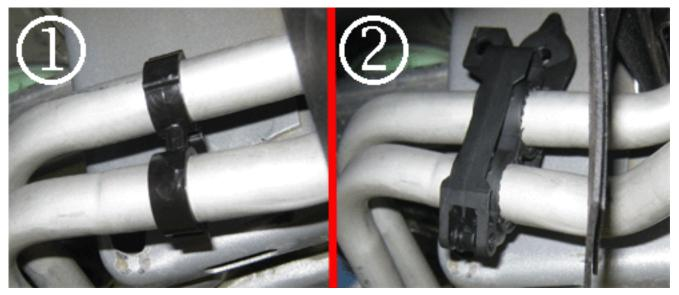
During the installation of the new line, replace the clips holding the lines (1) with the new clips (2) as illustrated above.
