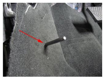
9. Lift the carpet back up, remove the rivets and use a punch to open the holes of the carpet to allow push pins through.
