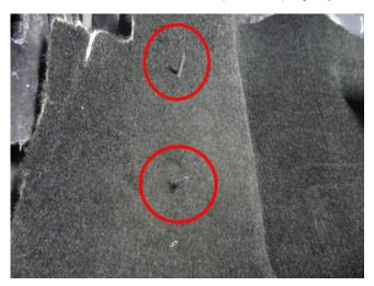
**8.** Push the carpet over the rivets and punch through the carpet as shown.
