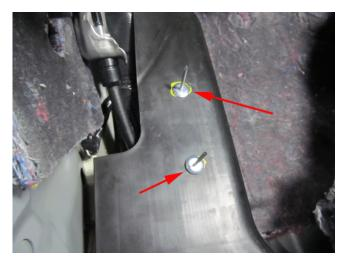
7. Place two rivets in the holes drilled and pull the carpet gently over the rivets.
