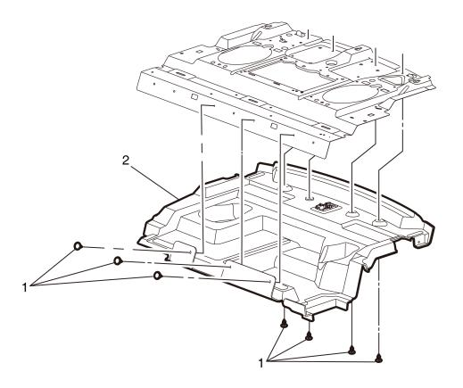
If you encounter a vehicle with the above concern, install the rear window panel stowage compartment cover. Refer to Rear Window Panel Stowage Compartment Cover Replacement in SI for installation instructions.
