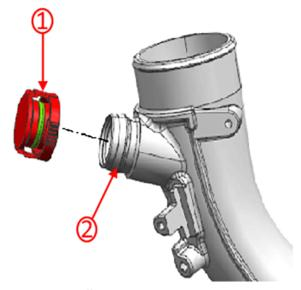
**5.** Install the block off plug (1) onto the turbocharger bypass port (2).
