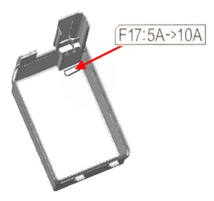
22. Install the UEC sticker onto the backside of the fuse block cover and in the owners manual under Engine Compartment Fuse Block.
