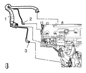
**4.** Remove and discard the Positive Crankcase Ventilation Hose/Pipe/Tube (1) and vacuum line. Refer to *Positive Crankcase Ventilation Hose/Pipe/Tube Replacement* in SI.
