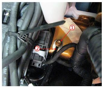
21. Install the PCV heater wiring harness ground (2) to an existing ground located at the frame stud (1).
