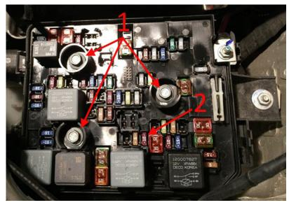
19. Position and snap the upper fuse block onto the base.
