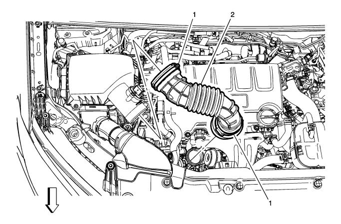
3. Remove and discard the air cleaner outlet duct (2) and resonator.
